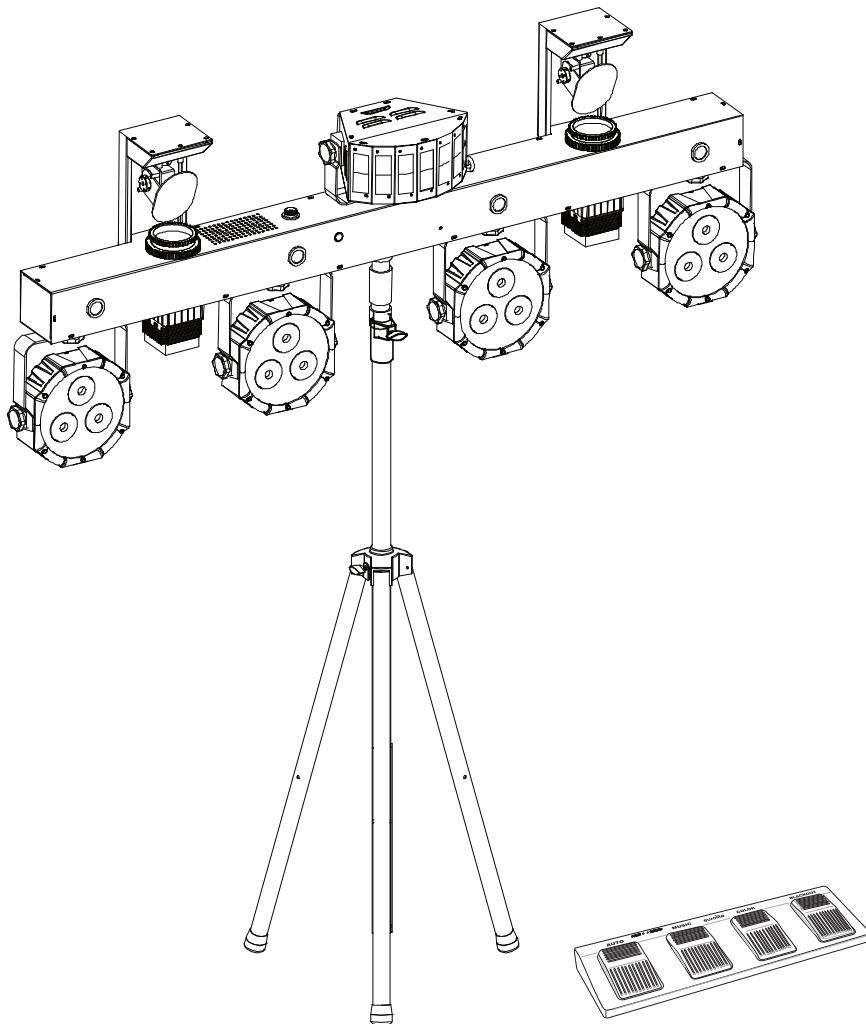
For mobile use, place the light set on a lighting stand via the TV spigot and fasten the fixation screw. Suitable stands can be found in chapter Accessories.
