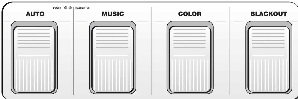
The optional wireless foot switch allows convenient control of the light set over a distance of up to 30 meters (line-of-sight). The foot switch will only work in stand-alone mode, it will not work in DMX or slave mode. The foot switch provides quick access to the show programs in automatic mode or sound control mode and a color mode with preset colors.
