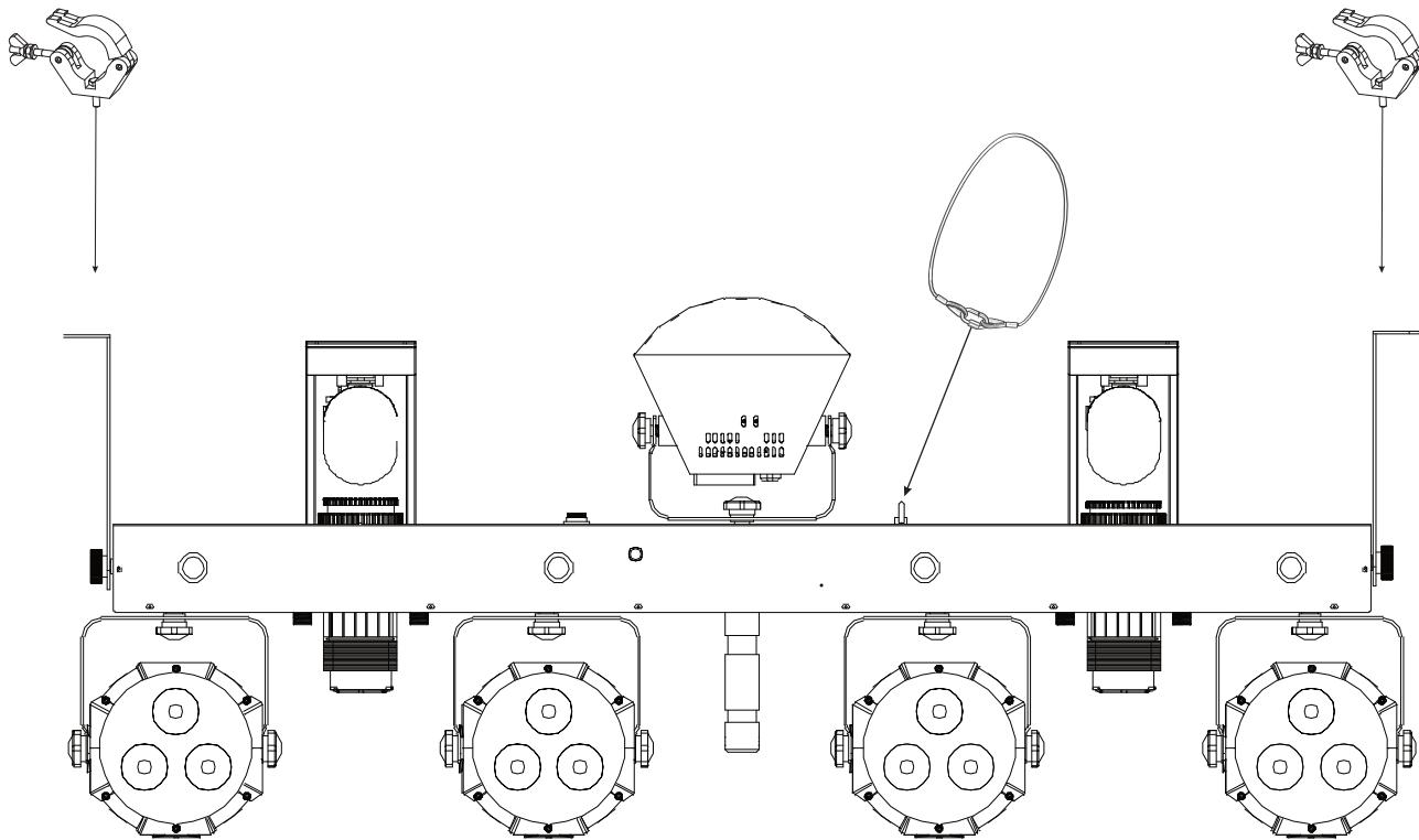
This device is designed for overhead rigging via the enclosed mounting brackets and may be fastened to a truss or similar rigging structure. The device must never be fixed swinging freely in the room.
